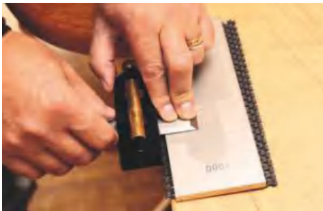
▲ Blade projection is sufficient to allow easy backing off while still in the guide
